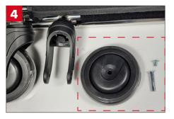
When both parts of the screw are removed, you can take OFF the wheel. All parts MUST be changed.
