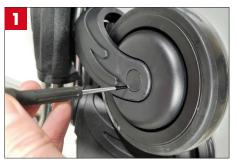
Insert the flathead screwdriver DELICATELY into the gap between the protective cover and the plastic wheel support. GENTLY action = No damage!
